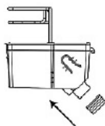
Install the water container on the door. Ensure that the seal ring has been inserted into the water valve before. Hold both sides of the water container tightly and install the container at an angle of 45°.
