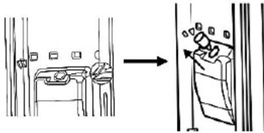
Clean all parts (water tank, cover, seal ring and water valve) using hot soapy water, then rinse thoroughly and dry.
