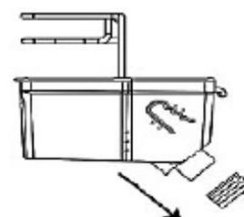
ter valve should raise and then be removed by hand at an angle of 45°.
